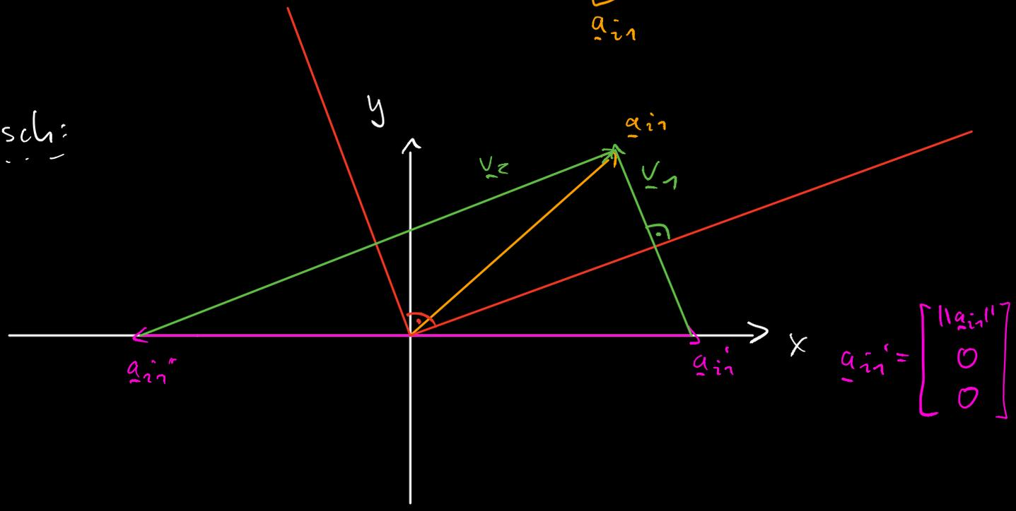
$$\underline{a}_{in} = \begin{bmatrix} 2 \\ 2 \\ 1 \end{bmatrix}, \|\underline{a}_{in}\| = \sqrt{4+4+1} = 3, \underline{e}_1 = \begin{bmatrix} 1 \\ 0 \\ 0 \end{bmatrix} \Rightarrow \underline{a}_{in}' = \begin{bmatrix} 3 \\ 0 \\ 0 \end{bmatrix}$$
